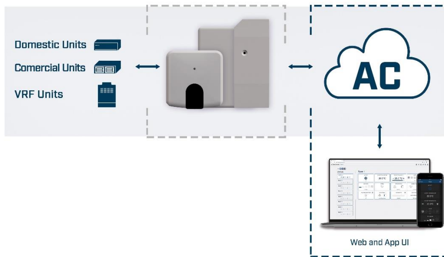
Figure 1.1 AC Cloud Control integration.
