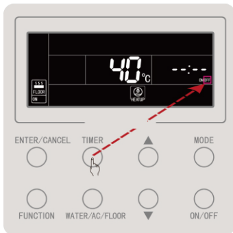
Press the "TIMER" button to switch to the setting of floor heating power-off time
