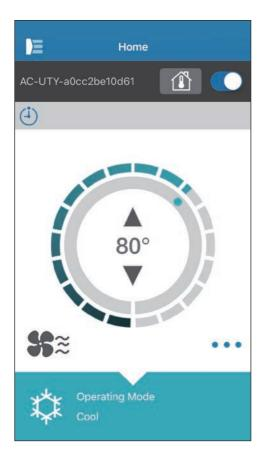
By tapping ▲▼ icons or by tracing the outer rim (circle) of the current temperature, you can set the temperature of your choice.
