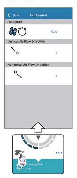
By selecting each item as shown on the screen, you can set the fan speed and airflow direction. For detailed information on each setting, refer to the operating manual of the air conditioner.
