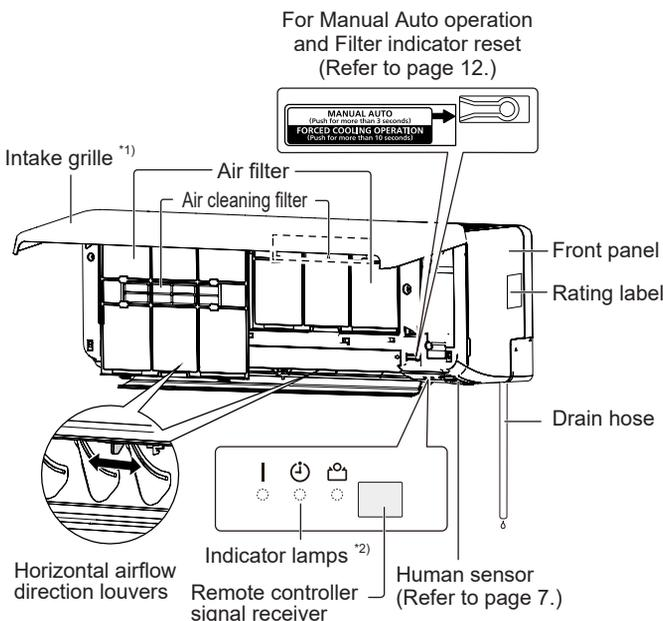
\*1) Before starting operation, make sure that the intake grille is closed completely. Incomplete closing may affect the proper function or performance of the product.
