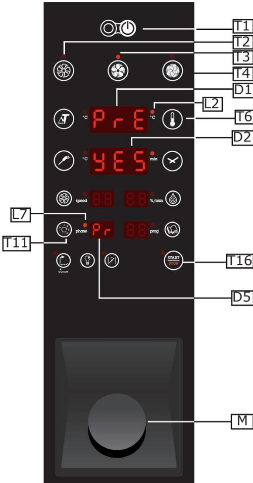
Modify the state of display **D2** pressing the knob **M** (it will pass alternatively from yes to no) and confirm selection by pressing the key **T11**.
