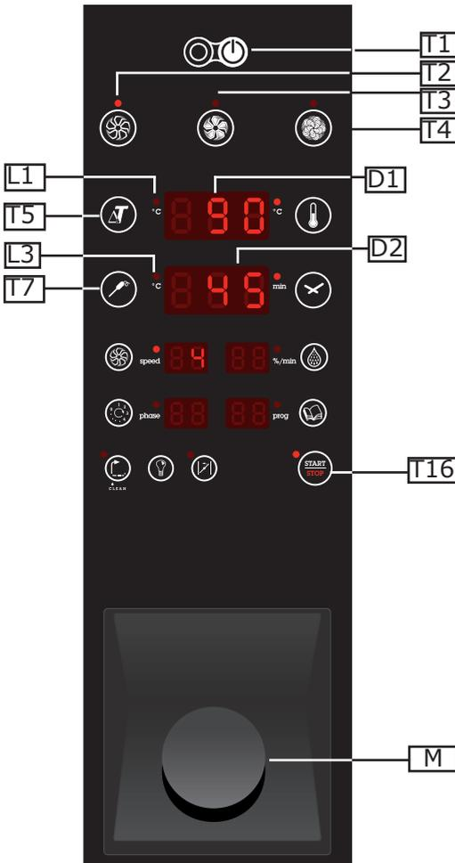
Set the temperature value at the heart of the product by acting on the **M** knob and confirm the selection by pressing the **T7** key or the **M** knob of the encoder. Continue with the definition of the ulterior cooking phase parameters according to the chosen type of cooking. Press the **T16** Start key to start cooking.
