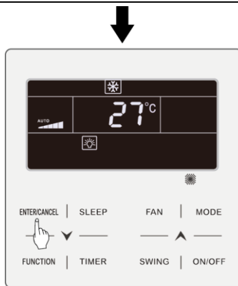
Fig.6.15 Turn on Filter Clean Reminder Function in Celsius
