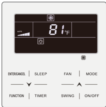
Fig. 6.3 Interface of On status in Fahrenheit
