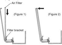
5. Push in both sides and the center of the intake grille.
