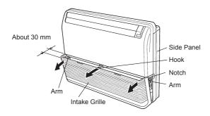
2. Pull the air filters upward to remove them. Push the air filter handles away from the intake grille in direction [A], then pull out the air filters.
