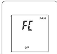
If no buttons are pressed within 30 seconds after the "FC" status is displayed, the system returns to the original clock display. In this case, start again from step 1.
