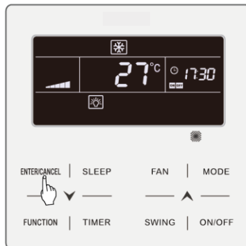
Fig. 4.7 Unit On/Off time setting in unit On status in Celsius
