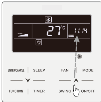
Fig. 4.7 Unit On/Off time setting in unit On status in Celsius
