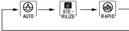
Figure 4.4 Function Switchover in Preset Mode and Night Mode
