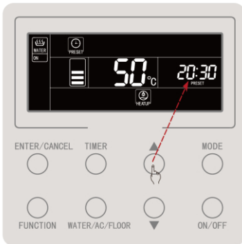
Press the "▲" or "▼" button to set the preset time for water heating
