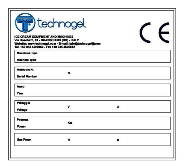
When ordering spare parts and requesting technical assistance, please supply the main information given on the serial plate to precisely identify the machine: Type, Serial n. and Year.
