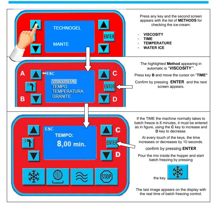
The entered and confirmed value 8.00 remains in the memory and will appear each time the time Method is recalled.
