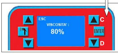
If the shown value of viscosity is inadequate, increase or decrease using the **C** or **D** key and then press **ENTER** to confirm.
