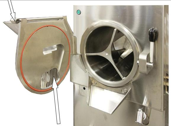
Do not tamper with or modify the output safety grid of the ice-cream.
