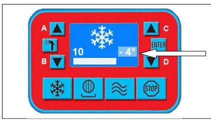
The last image appears on the display with the real time of batch freezing control.
