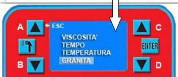
Choose the WATER ICE **Method** by moving the white cursor on the word "WATER ICE" by pressing the **A** or **B** keys.
