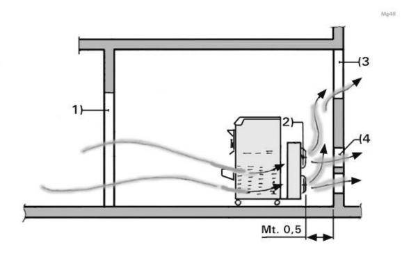
As can be seen in the diagram, the air entering through door (1) is sucked in and heated during condensation from the ventilators (2). It is then pushed towards the window (3) from which it exits.
