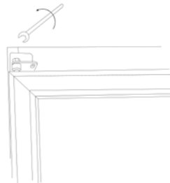
8. Tighten the top hinge pin.
