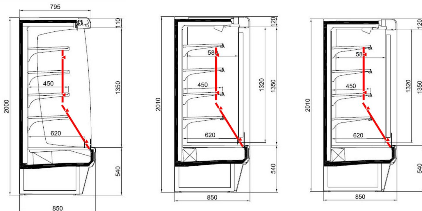
**N.B.:** Counter operation is guaranteed in the climate conditions indicated on the serial number plate and according to standards ISO 23953-2 if loaded evenly and not beyond the conforming loading line on each counter.
