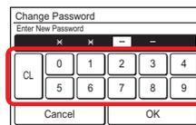
When the new password is entered and the [OK] is touched, after the setting change screen is displayed, the display returns to the "Password Setting" screen.
