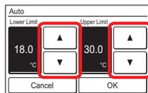
When the [OK] is touched, the display returns to the “Setting” screen. If the [Back] on the “Setting” screen is touched, the display returns to the “Temp. Range Setting” screen.
