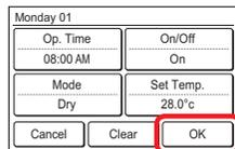
When the [OK] on the screen of (5) is touched, the display returns to the screen of (3).
