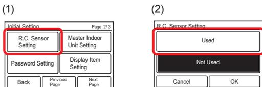
When the [OK] is touched, after the data is transmitted to the indoor unit, the display returns to the "Initial Setting" screen.
