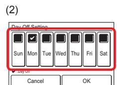
When setting is complete, touch the [OK]. After the setting complete screen is displayed, the display returns to the "Weekly Timer Setting" screen.
