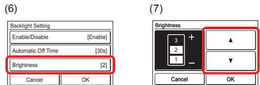
When the [OK] is touched, the display returns to the "Backlight Setting" screen.
