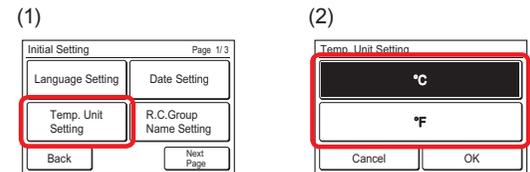
When the [OK] is touched, after a setting change screen is displayed, the display returns to the “Initial Setting” screen.
