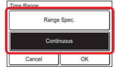
When the [OK] is touched, the display returns to the "Time Range Setting" screen. When the [Continuous] is selected, go to (14).
