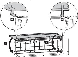
4 Press 4 places on the intake grille to close it completely.
