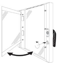
The door glass can be cleaned externally and internally. For this purpose, turn the stop holding the internal glass in position clockwise and, once the glass is opened, clean it with suitable detergent.
